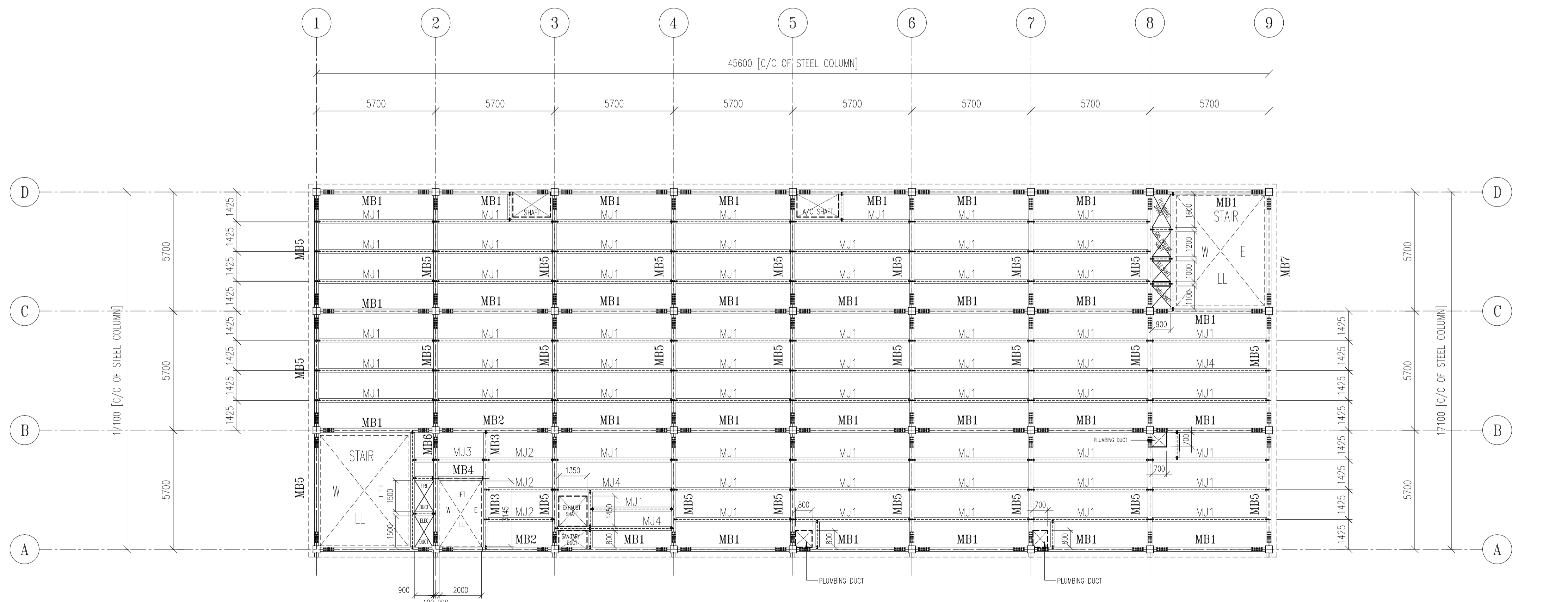
FIRST FLOOR FRAMING PLAN AT (+) 5.000M. LVL.]
